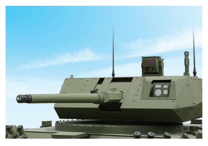
The TEBER-30/35 RCT is a remote controlled turret designed to be installed on wheeled and tracked armoured vehicles and equipped with a medium calibre automatic cannon, an advanced target detection and a fire control system. Unlike conventional turrets, remote controlled turrets do not have any basket structure and thus the extra available interior space provides a significant advantage to the user.
